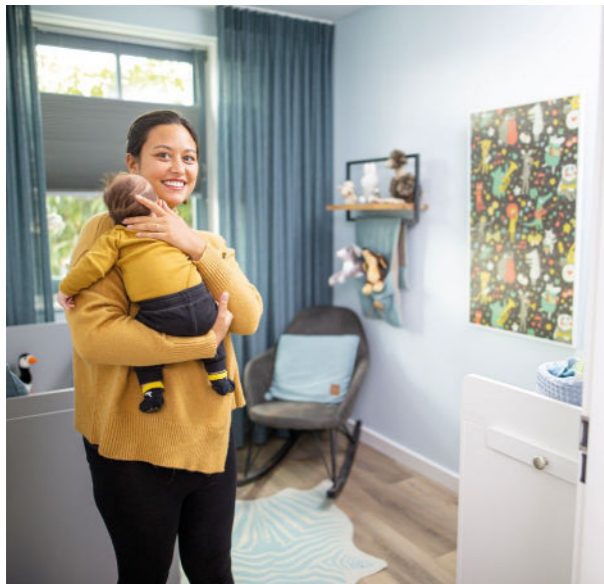
The children's room has a size of 12 m 2 . Due to the good insulating properties of the room, a 600 watt picture heater is used. The heater was printed with a customised motif.
